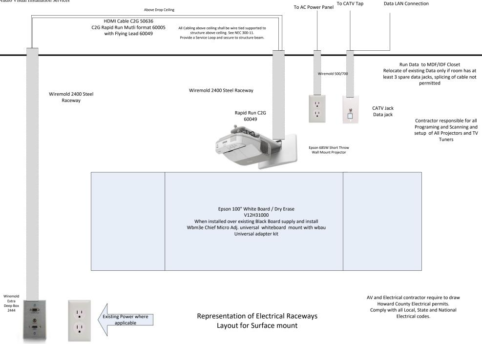
Low AV Jack to be located with in 25' of Projector to the Left or Right of Projection surface, with in proximity of existing Power receptacle. VGA 3.5 HDMI C2G # 60145
